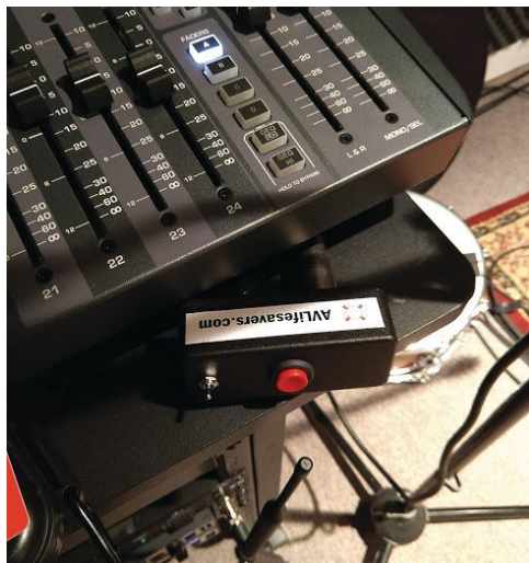
The Mini Mic Switch that adds a talkback button to a console.
